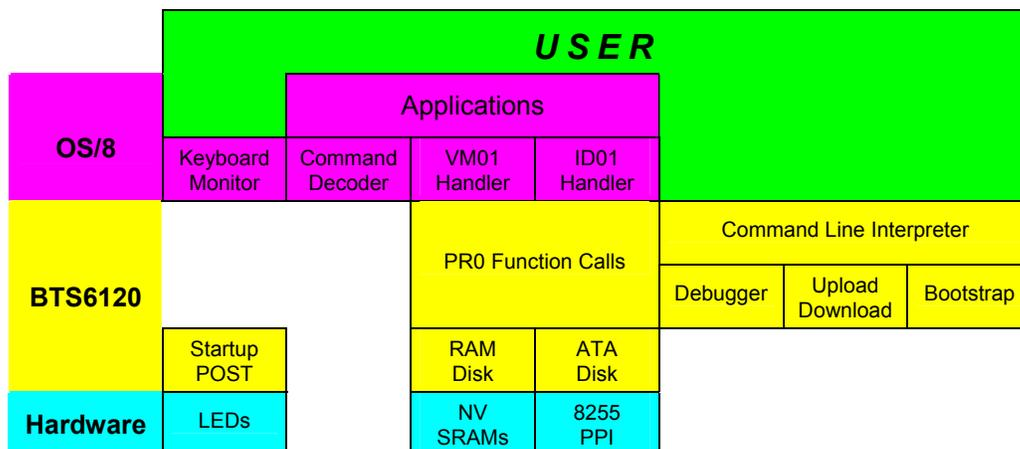
Figure 6 - SBC6120 Software Architecture
